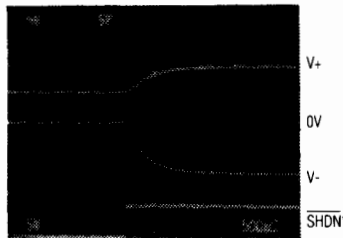
V_{+} , V_{-} WHEN EXITING SHUTDOWN ( 1\mu\text{F} CAPACITORS)
